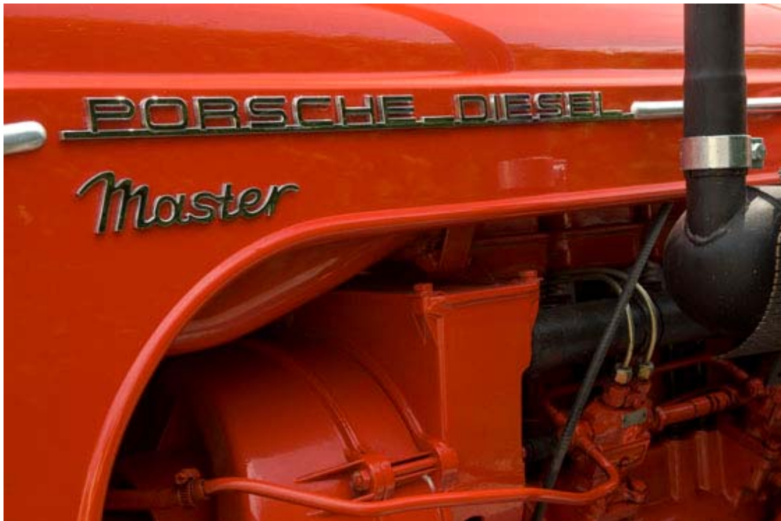
Porsche 3 litre air cooled diesel engine. Ca. 1960
